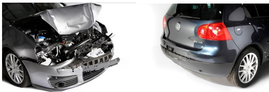
Figure 7: Vehicle damage – 16 km/h Underride
