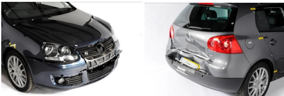
Figure 6: Vehicle damage – 16 km/h Engagement
